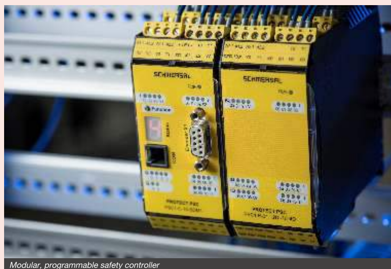
Modular, programmable safety controller
