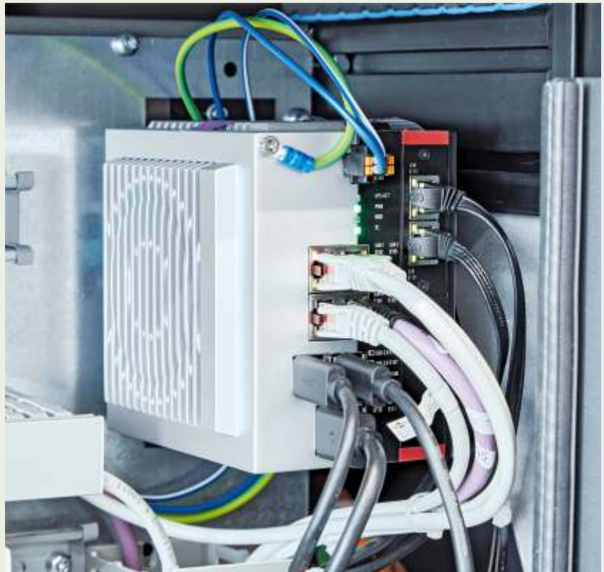
The high-performance C6032 ultra-compact Industrial PC controls all machine and process sequences with numerous TwinCAT software functions, such as TwinCAT Vision. © Beckhoff
