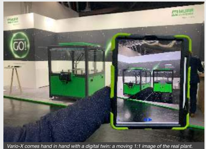
Vario-X comes hand in hand with a digital twin: a moving 1:1 image of the real plant.
