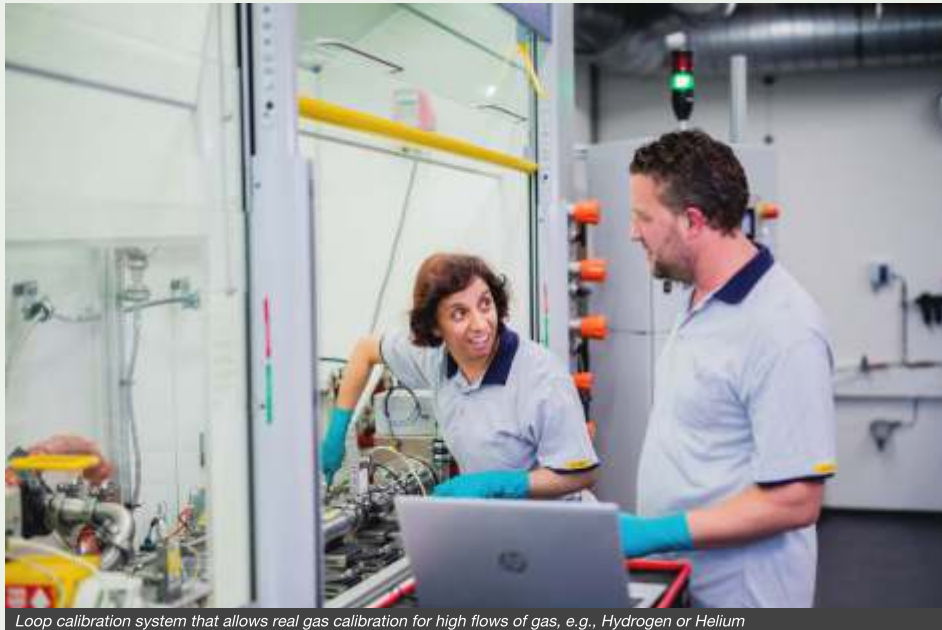
Loop calibration system that allows real gas calibration for high flows of gas, e.g., Hydrogen or Helium
